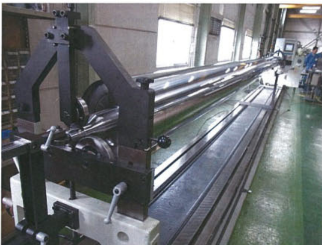
Figure 4 \phi 350 \times L9,200 mm Roller Testing
